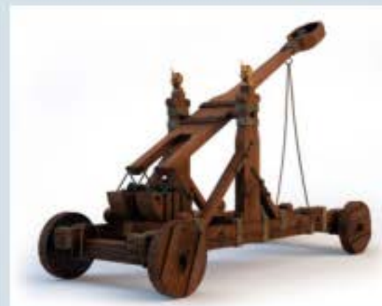
FIGURE 2.3.2 The formidable counterweight trebuchet first came into use in the 12th century and was used by armies to fling projectiles at enemy fortifications
