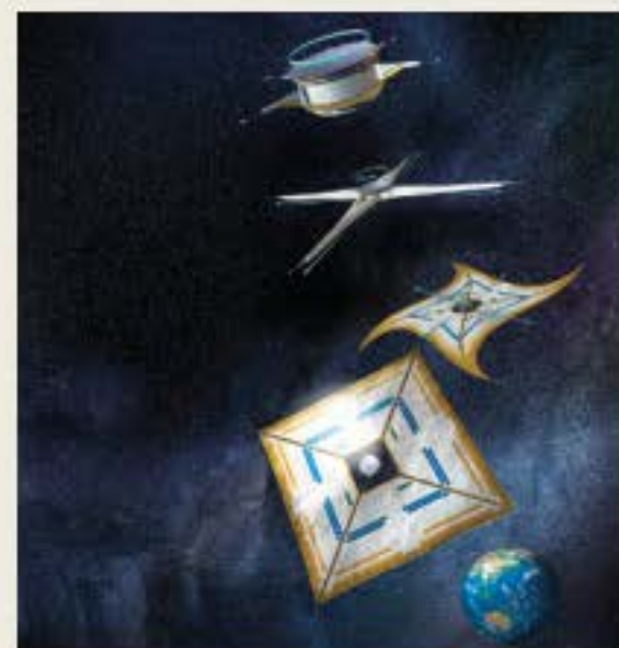
FIGURE 7.6.10 The IKAROS spacecraft is the first interplanetary spacecraft to use solar-sail technology.
