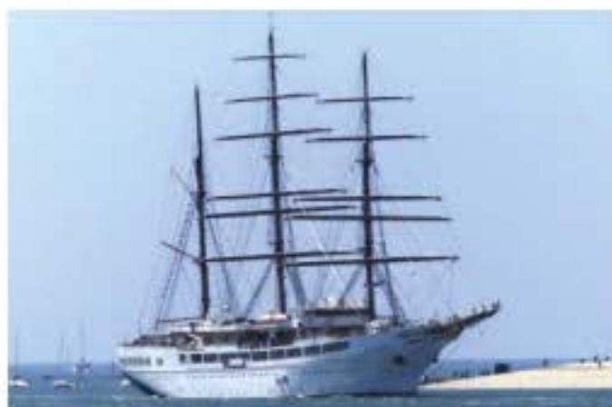
FIGURE 3.3.2 To keep each mast in rotational equilibrium in relation to its base, the stainless steel cables (stays) attached to it must provide opposing torques on the mast.
