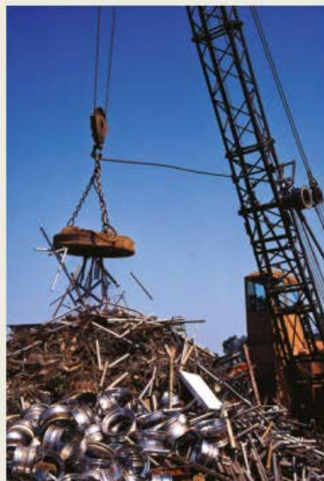
FIGURE 5.1.18 A large electromagnet is used to lift waste iron and steel at a scrapyard. Valuable metals such as these are separated and then recycled.
