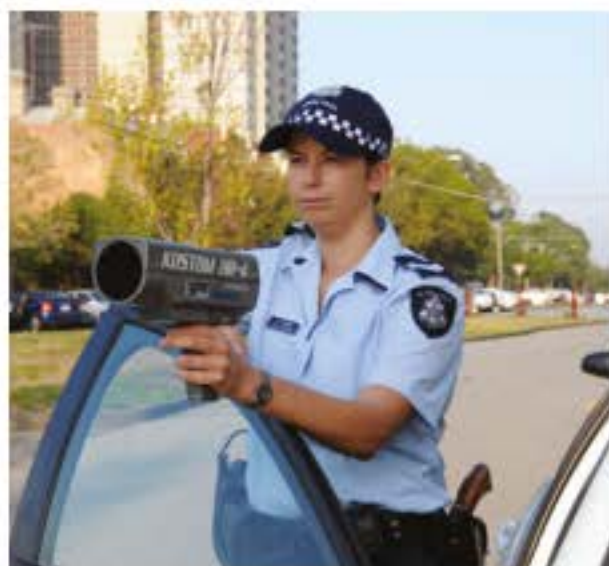
FIGURE 10.2.2 To avoid a systematic error, make sure that you are using measuring equipment correctly. Laser speed guns, for example, need to be placed on a stationary support so the aim point is held on a single target point for the duration of the read.
