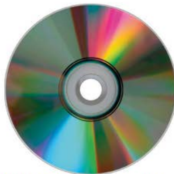
FIGURE 7.1.20 Information on a CD or DVD is stored using a tight spiral of bumps or pits. These small structures are created by a laser and are of the size of a wavelength of light. This means these structures are small enough to cause light to diffract.
