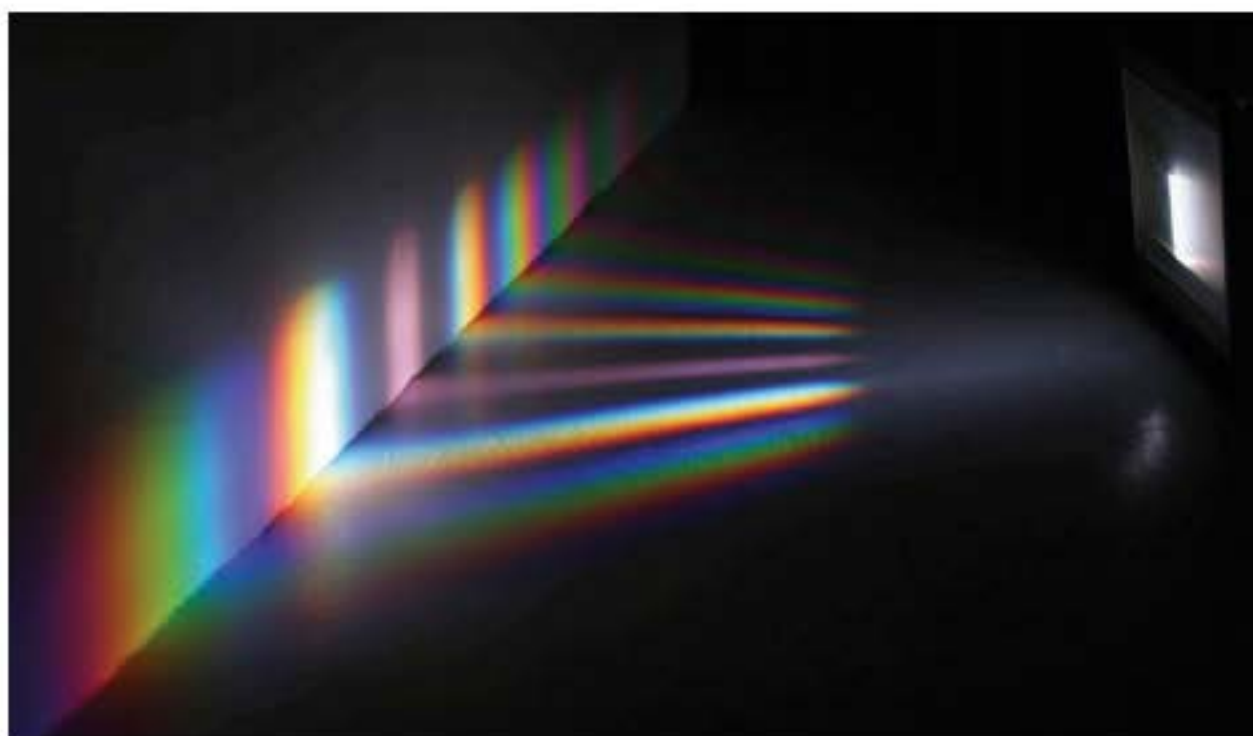
FIGURE 7.1.23 A diffraction grating disperses white light into a series of coloured spectra.
