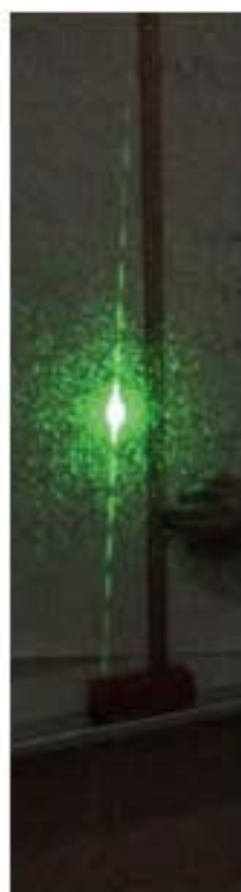
FIGURE 7.1.19 The interference pattern obtained from a cotton thread.
