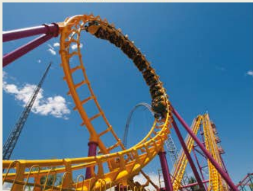
FIGURE 2.6.7 The thrill seekers on this rollercoaster ride don't fall out when upside down because the centripetal acceleration of the cart is greater than 9.80 \text{ m s}^{-2} down.
