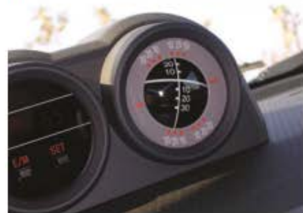
FIGURE 3.2.4 (a) The car on the incline is in stable equilibrium, while the heavily laden truck on the same incline could topple. The weight vector is outside the lower point of support for the truck, so there is no reaction force from the road to the higher wheel. (b) Modern four-wheel drives and tractors have inclinometers to warn the driver if the vehicle is in danger of tipping.
