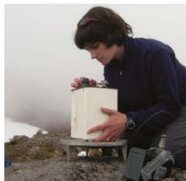
FIGURE 1.2.5 A gravimeter can be used to measure the strength of the local gravitational field.
