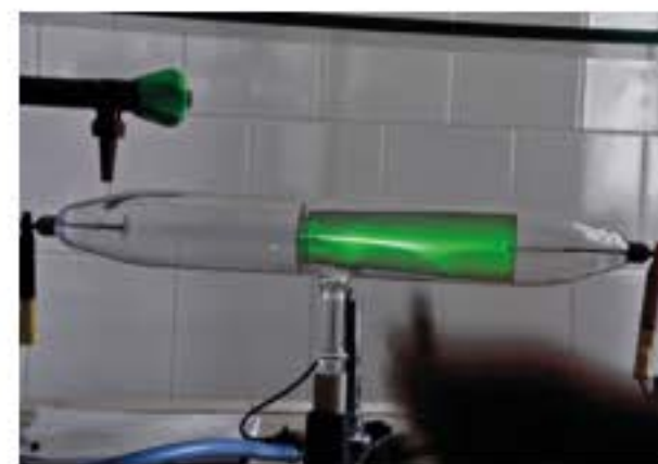
FIGURE 5.2.2 The electron beam of a cathode ray tube is deflected by a magnet in the foreground.
