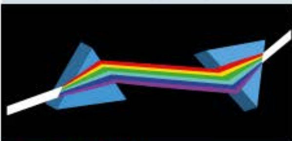
FIGURE 7.1.16 Newton's double prism experiment showed that white light is made up of its component colours.
