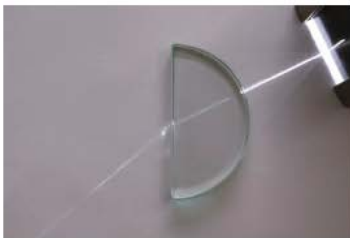
FIGURE 7.1.7 Light refracts as it moves from one medium (i.e. the semicircular glass prism) into another (i.e. air), causing a change in direction.
