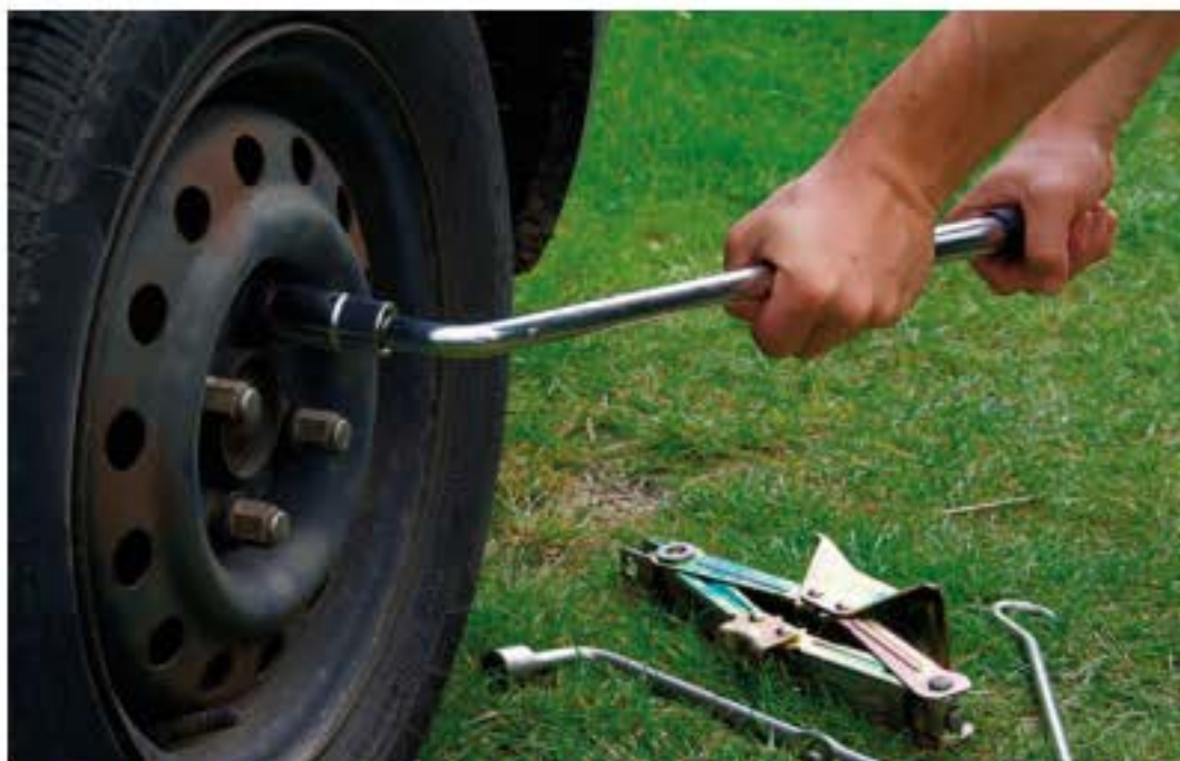
FIGURE 3.1.8 Loosening the wheel nuts with an extended handle spanner will increase the torque on the nut.
