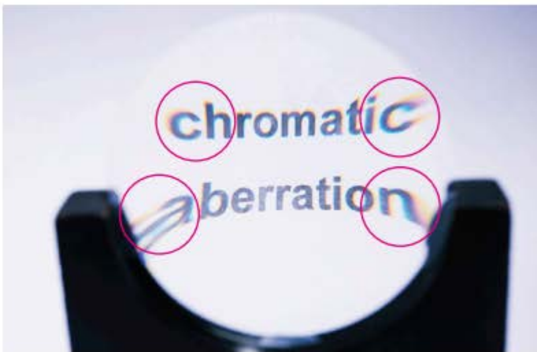
FIGURE 7.1.17 Chromatic aberration causes the coloured fringes that can be seen in the circled regions in this image.
