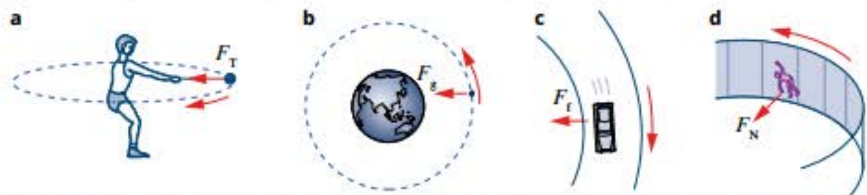
FIGURE 2.4.6 (a) In a hammer throw, tension in the cable provides the centripetal force. (b) For planets and satellites, the gravitational attraction to the central body provides the centripetal force. (c) For a car on a curved road, the friction between the tyres and the road provides the centripetal force. (d) For a person in the Gravitron ride, it is the normal force from the wall that provides the centripetal force.
