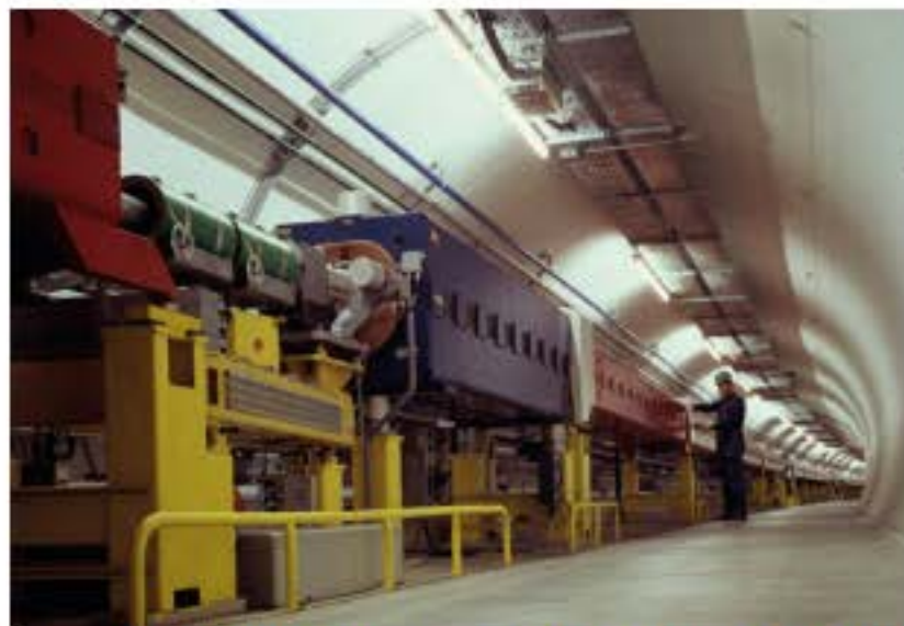
FIGURE 9.3.11 The tunnel of the Super Proton Synchrotron (SPS) particle accelerator at CERN, the European particle physics laboratory outside Geneva.
