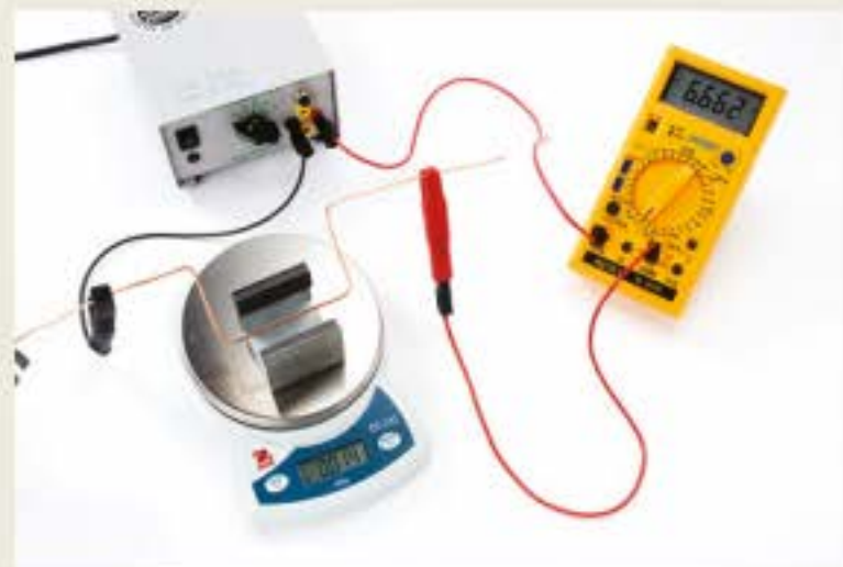
FIGURE 5.3.2 A current balance is used to measure the interaction between an electric conductor and a magnetic field. The relationship between force, current and conductor length can be shown.
