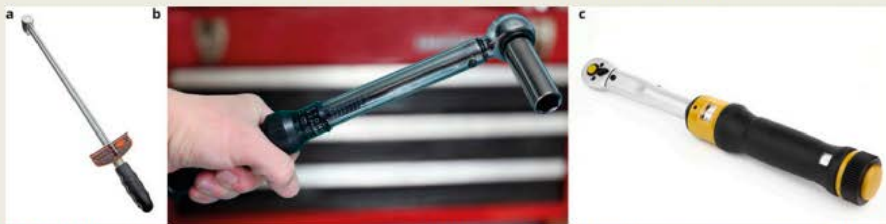
FIGURE 3.1.13 Three types of wrenches commonly used to measure the torque applied to a nut or bolt: (a) beam torque wrench, (b) click-type torque wrench, (c) digital torque wrench.
