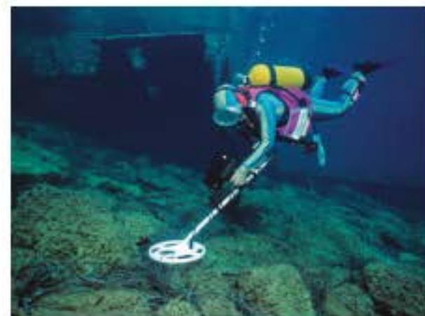
FIGURE 6.3.1 A diver using a metal detector. If a metal object is found underneath the coil of the detector, an emf will be induced, which creates a current that will affect the original current. The direction of the induced current is predicted by using Lenz's law.
