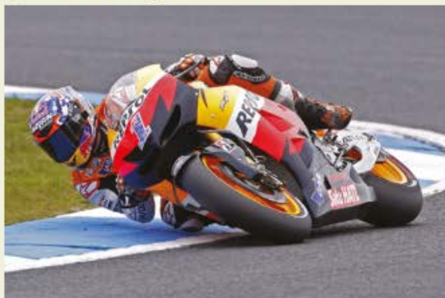
FIGURE 2.5.7 Australia's Casey Stoner won the 2012 Moto GP championship. Here he is leaning his bike as he takes a corner at Phillip Island. Leaning into the corner enables him to corner at higher speeds. In fact, the bike would go out of control if he did not lean it.
