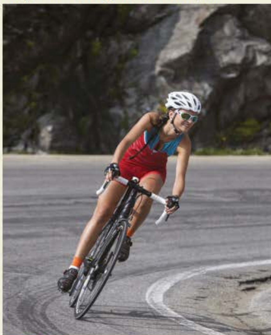
FIGURE 2.5.8 The forces acting as the rider turns a corner are the weight, F_g , the normal force, F_N , and the friction, F_f , between the tyres and the road. The friction supplies the unbalanced force that leads to the corner-turning motion.
