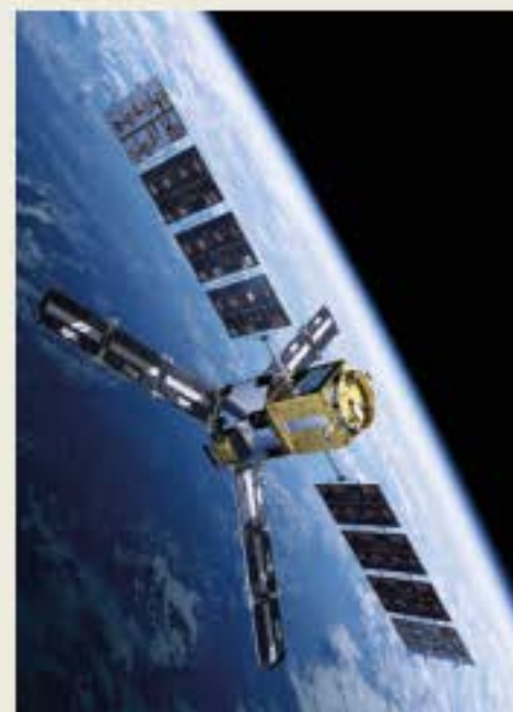
FIGURE 1.1.16 A low-orbit satellite called the Soil Moisture and Ocean Salinity (SMOS) probe was launched in August 2014. Its role is to measure water movements and salinity levels on Earth as a way of monitoring climate change. It was launched from northern Russia by the European Space Agency (ESA).
