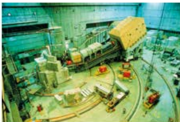
FIGURE 9.3.3 The End Station, an experimental hall at the Stanford Linear Accelerator Center, contains three giant particle spectrometers that detect particles of different energies and scattered at different angles.
