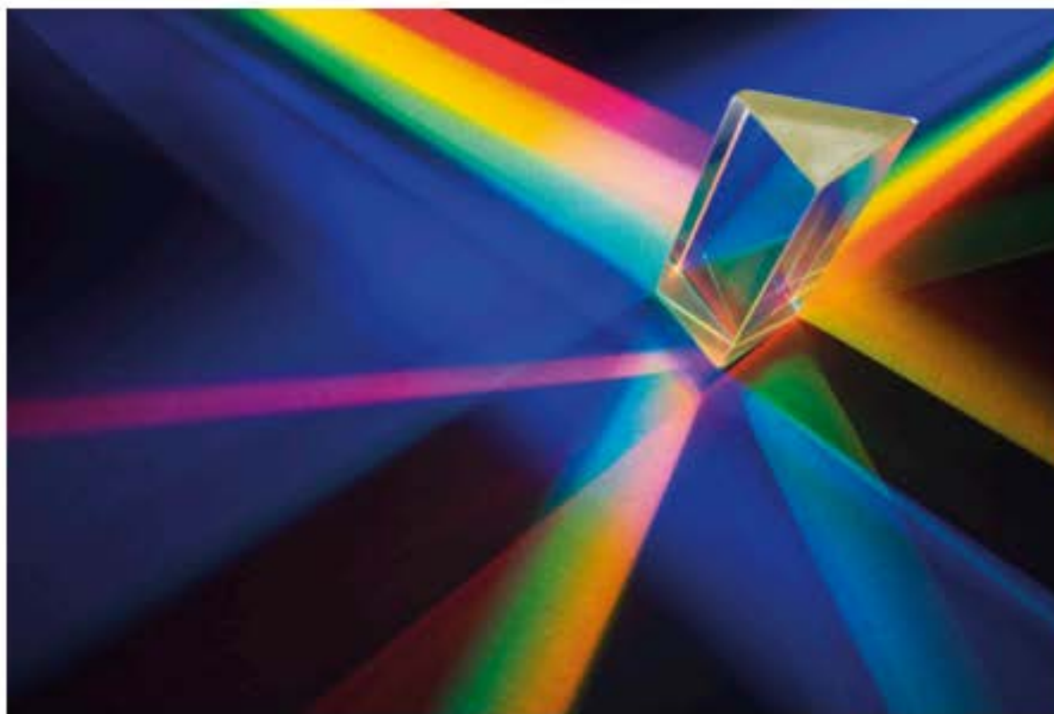
FIGURE 7.1.1 The wave model of light can explain the phenomenon of the dispersion of light into its component colours.
