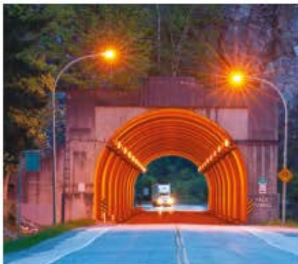
FIGURE 7.5.9 Sodium vapour lamps are sometimes used as street lights and have a distinctive yellow colour due to the yellow wavelengths of the sodium emission spectrum.
