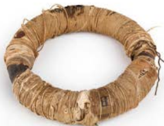
FIGURE 6.1.1 Michael Faraday's original induction coil. Passing a current through one coil induces a voltage in the second coil by a process called mutual inductance. This coil is now on display at the Royal Institution in London.
