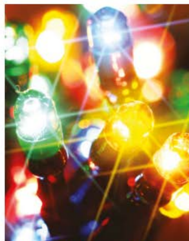
FIGURE 7.5.12 LEDs can be produced in virtually every visible and near-visible colour.
