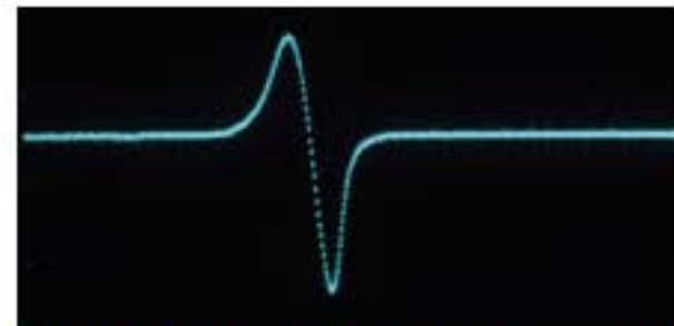
FIGURE 6.2.1 Oscilloscope trace from an electric coil, showing the voltage across the coil as a magnet is dropped through it.
