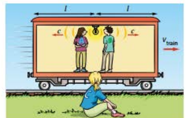
FIGURE 8.1.6 Amaya and Binh see the light take the same time, \frac{l}{c} seconds, to reach the front and back walls.
